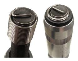
Mount the 5/8"-18 threaded insert onto the installation tool and thread the tool collar over the insert, taking care to ensure that the insert tang is properly engaged as shown
