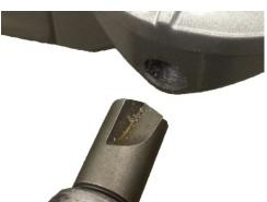
Countersink the hole entrance to a diameter of 11/16" using a 3/4" 120° Countersink
