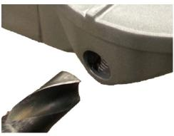
Expand the existing hole using a 41/64" diameter drill to a depth of 1-1/2"
