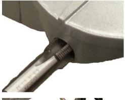
Cut new screw threads into the drilled hole using the appropriately sized tap for a 5/8"-18 threaded insert
