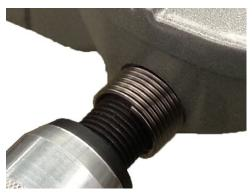
Install the 5/8"-18 threaded insert using the insertion tool by screwing the insert into the tapped hole
