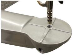
Clean the hole using a shop rag or compressed air to remove all metal chips
