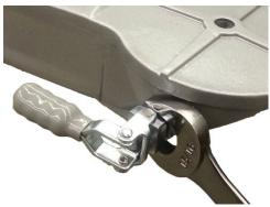
Adjust Quick Release Clamp as necessary and tighten Jam Nut using 1" Wrench
