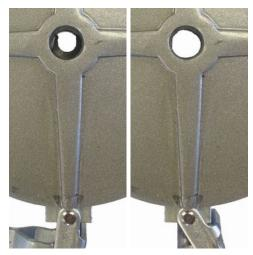
View pin insertion hole to check for proper alignment and clearance.
