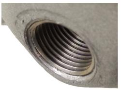
After installation, the threaded insert should be about 1/2-turn past flush with the surface as shown
